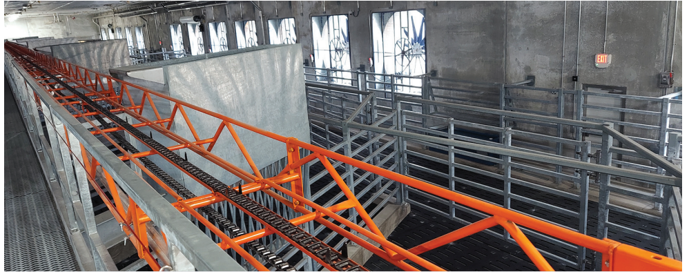
The new barn features automation to assist employees. Here you'll see an orange conveyor. This helps employees move hay bales throughout the barn so they can be dropped into feeders for the cattle to access.
